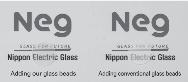
Appearance of 0.5mm-thick resin plates containing 30vol% glass beads
